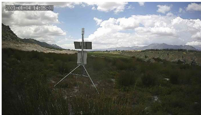
Figure 11. Picture taken by the humidity stack camera towards the end of the humidity rally, indicated with the red dot on the left of Figure 10. Clouds are starting to form. Temperature: 27.67 ^{\circ}C ; relative humidity: 50.5%; wind: 3.26 m/s N; GHI: 753.83 W/m^2 .
