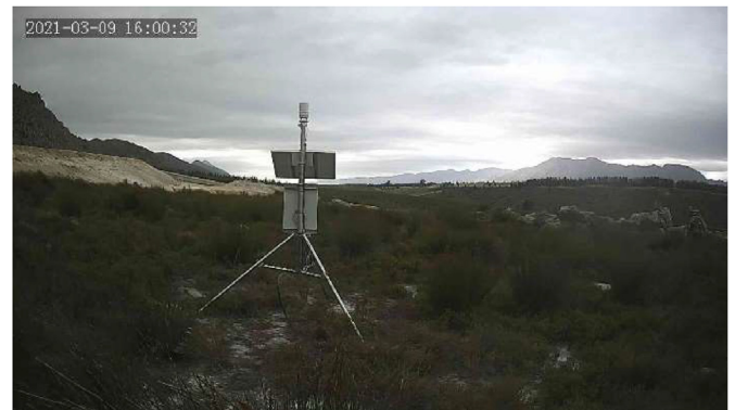
Figure 12. Picture taken by the humidity stack at the point indicated by the red dot on the right of Figure 10. Cloud cover is starting to form. Temperature: 15.1 ^{\circ}C ; relative humidity: 62.9%; wind: 8.58 m/s N-E; GHI: 65.87 W/m^2 .
