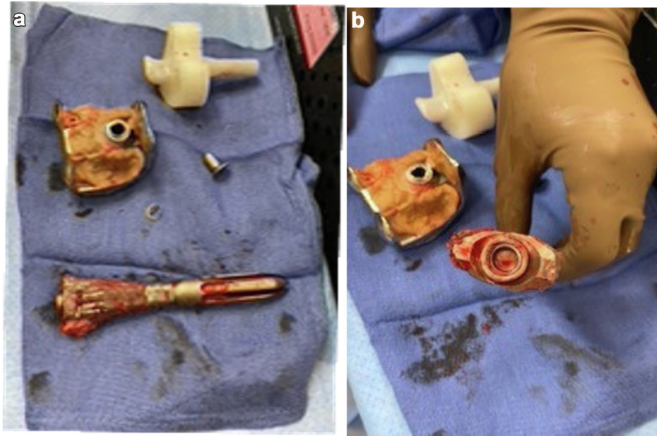
Figure 4. Extracted implant showing fractured morse.
