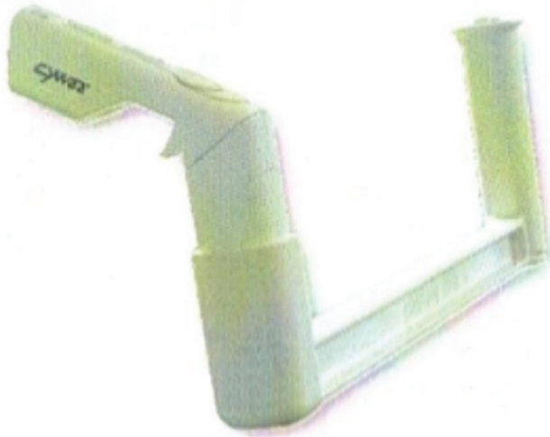
Fig. 2. Custom controller attached on the custom-made handlebars (AbleX, Auckland, New Zealand) with one end for the paretic hand and the other end for non-paretic hand.
