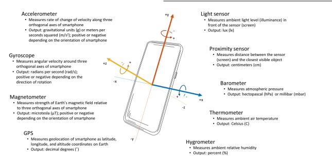
**Fig. 6** Overview of standard smartphone sensors. Inertial sensors (accelerometer, gyroscope, and magnetometer) provide measurements with respect to the three orthogonal axes (*x*, *y*, *z*) of the body of the phone; the remaining sensors are orientation-invariant.
