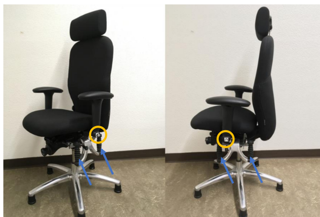
Figure 1. The dynamic swing system is located beneath the seat of the office chair (Haider Bioswing, Pullenreuth, Germany). The blue arrows indicate the location of two of four swinging elements. The yellow circles illustrate the location of the reflective markers at the base of the arm rest.
