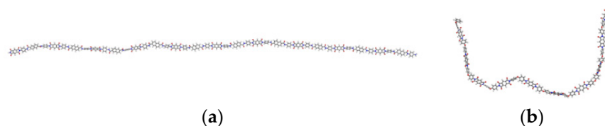
Figure 7. Single chain configurations (10 repeat units) of the (a) NAPPI and (b) Kapton [23].
