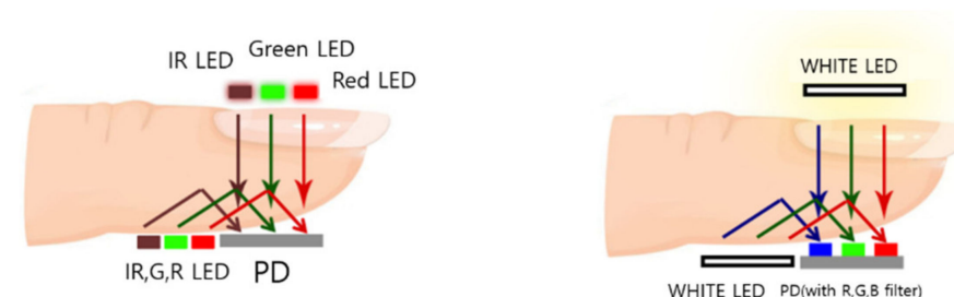
Figure 1. Example of LED–PD arrangement for HbA1c measurement.
