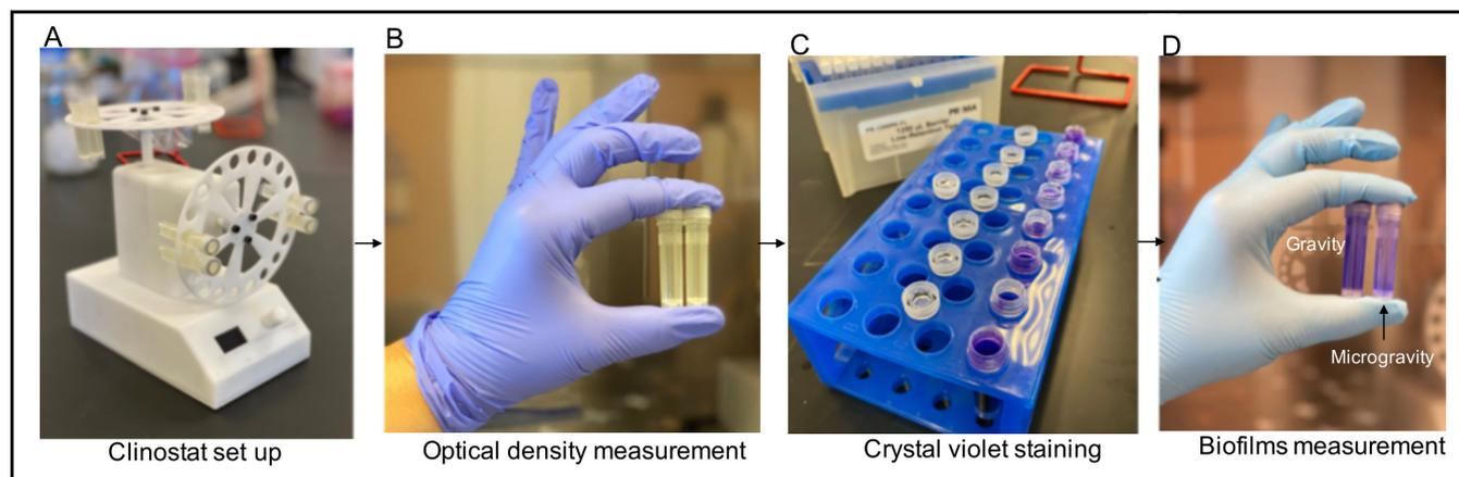
**FIG 2** Overview of *Escherichia coli* cultures growth under simulated microgravity showing the placement of growth vessels (tubes) on the EagleStat (A), a side-by-side comparison of cell density in a treatment and control tubes after a 24-h incubation at 30°C (B), the crystal violet staining step to measure biofilm development on the tubes (C), and the differential accumulation of biofilm biomass as a result of the treatment (D).
