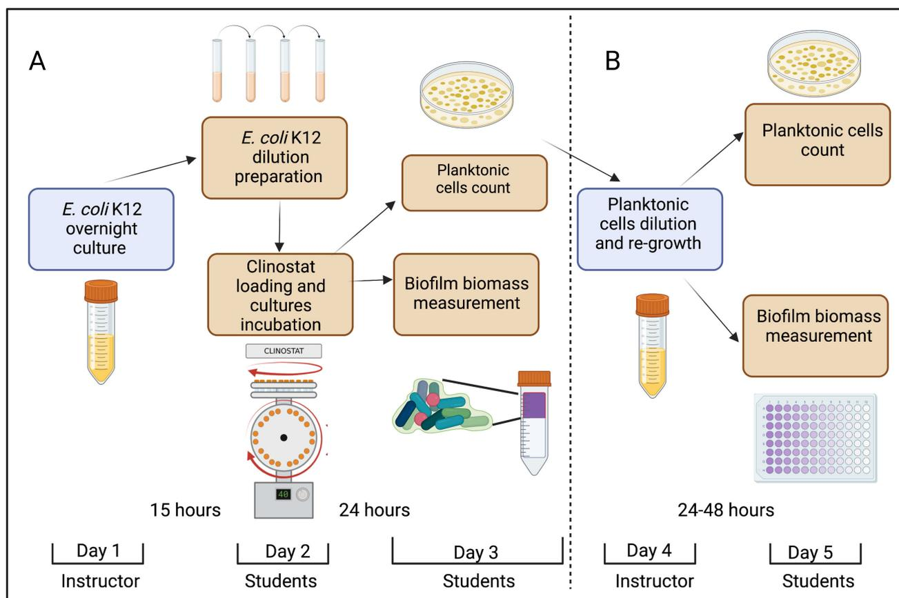
**FIG 1** Schematic of the activities required, by students and instructor, to study the effect of simulated microgravity on the growth and biofilm development in *E. coli* K12. This experiment is intended for undergraduate (A) and graduate students (B).
