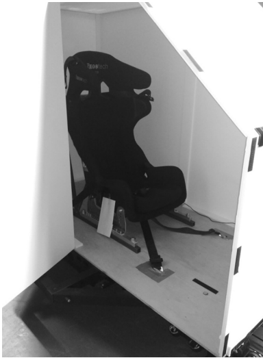
Figure 2. The inside of the cabin with the car seat and 5-point safety harness. The cabin prevented visual and haptic (via airflow) information on the occurring motion.
