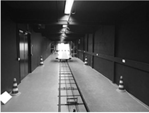
Figure 1. The motion platform and track. The full track was 40 m; however, in the present study, we exclusively utilized displacements of \pm 9 m.
