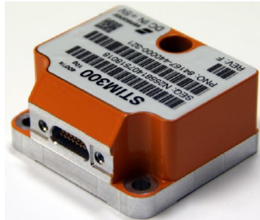
Figure 5. The IMU (STIM300) used that outputs instant angular velocity and acceleration at 200 Hz.
