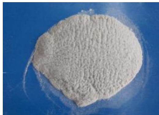
Figure 8. Optical images of the composite powder of wood flour, polyether sulfone (PES), and various amounts of 0.1% CNTs [84].
