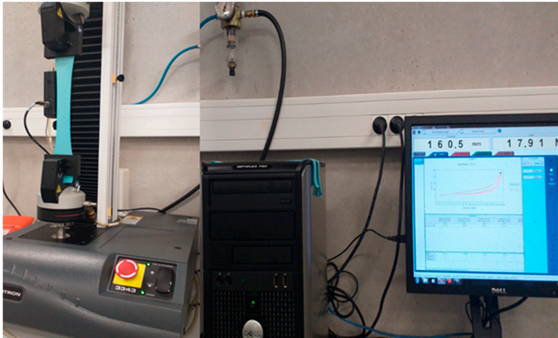
Figure 3. Strip tests for stretch-recovery measurement using an Instron 3334 Tensilemeter.
