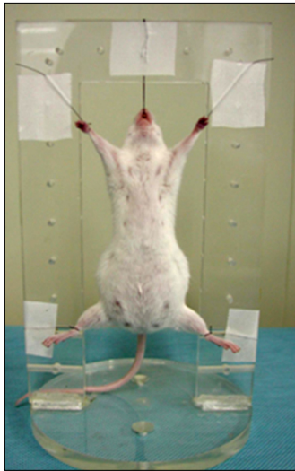
Fig. 2. Photograph of a pregnant mouse suspended in the rectangular positioner with surgical ties. Synchrotron radiation imaging was performed with the mouse in an upright position.
