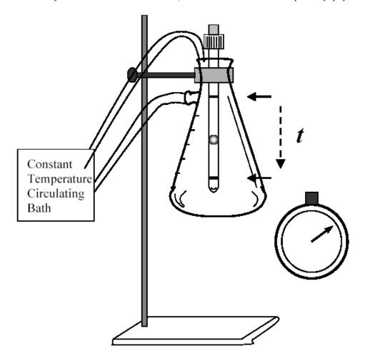
Fig. 4: Drawing of the setting used to measure viscosity. A Kitasatto flask containing the viscometer was filled with water and connected to a circulating bath with controlled temperature. The clamp holding the flask to the support could be rotated 180°C in order to duplicate the measurement of the time of ball descent.
