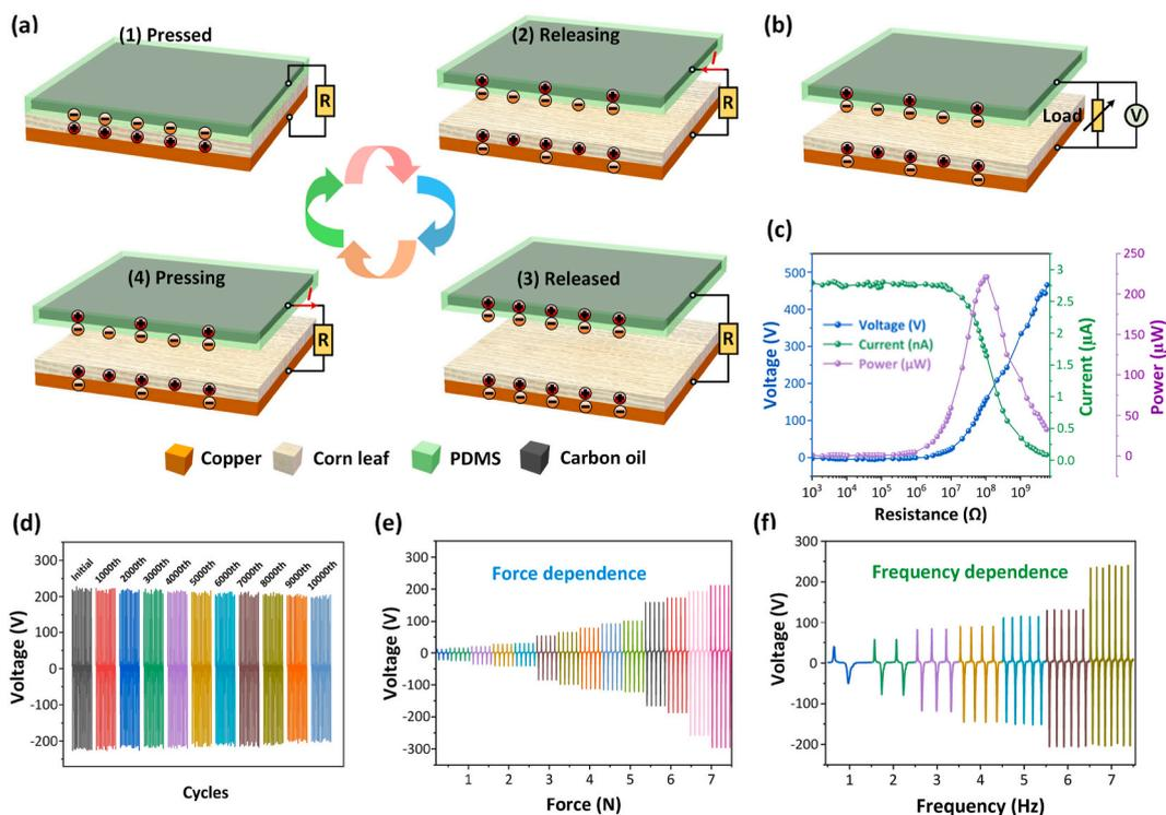
**Fig. 5.** (a) The operating mechanism of C-TENG for human motion energy harvesting. (b) The electrical output test circuit of C-TENG. (c) The relationship between electrical output of C-TENG and various load resistances. (d) The reliability testing of C-TENG. The output voltage of C-TENG under (e) different driving forces and (f) different driving frequencies.
