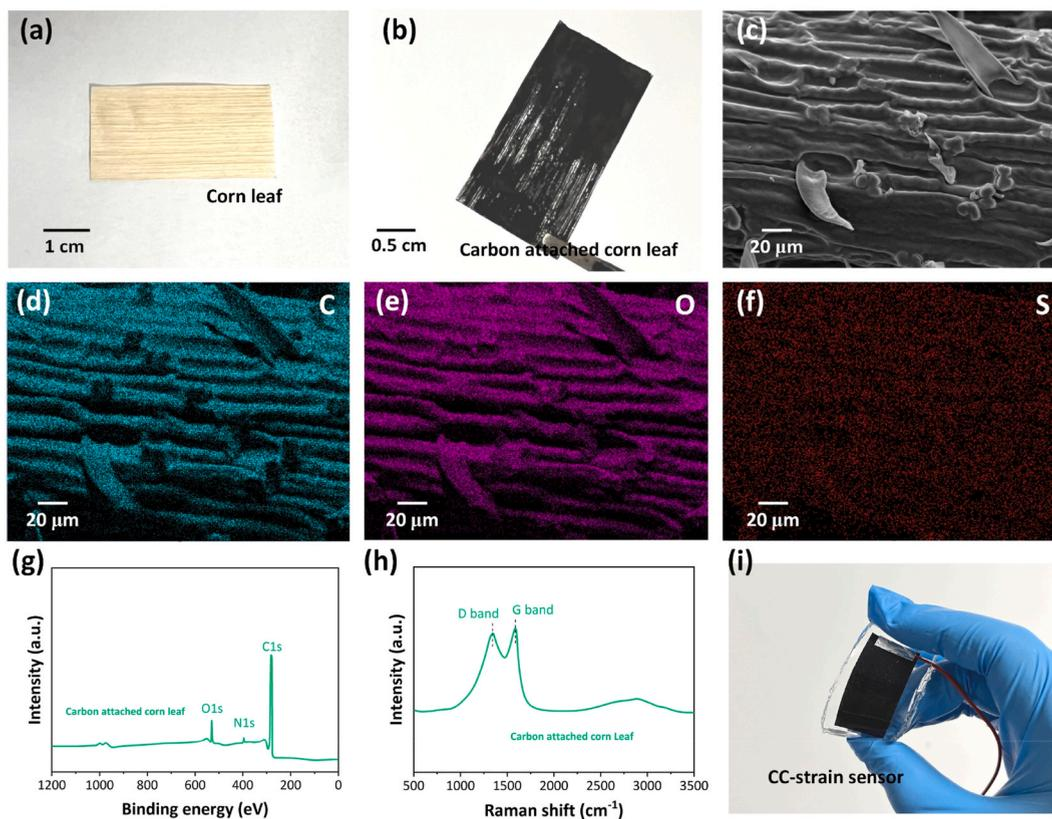
**Fig. 2.** The picture of (a) corn leaf and (b) carbon attached corn leaf. (c) The SEM image of corn leaf surface. (d–f) The element analysis of corn leaf. (g) XPS spectrum of carbon attached corn leaf. (h) Raman spectra of carbon attached corn leaf. (i) The picture of CC-strain sensor device.
