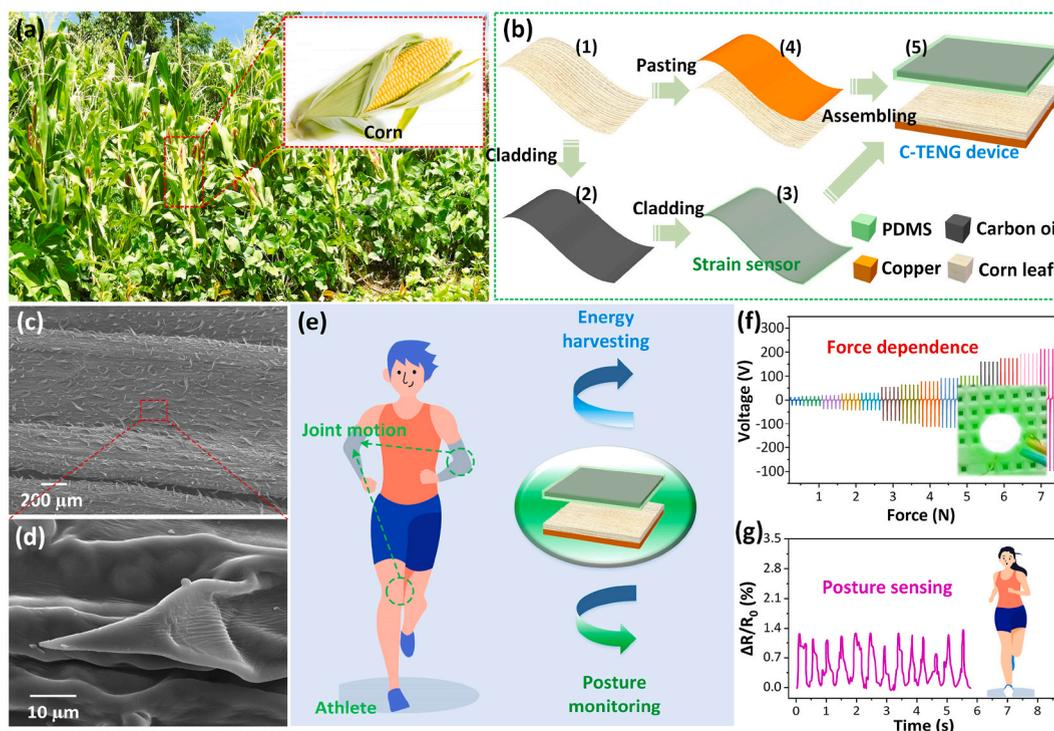
**Fig. 1.** (a) Photos of green corn field scenes (inset: photo of corn cob with corn leaves). (b1-b5) The manufacturing process of strain sensor and C-TENG device. (c, d) The SEM images of corn leaf surface. (e) The picture of athlete. (f, g) The energy harvesting and running posture monitoring application of C-TENG device and CC-strain sensor. (For interpretation of the references to colour in this figure legend, the reader is referred to the Web version of this article.)
