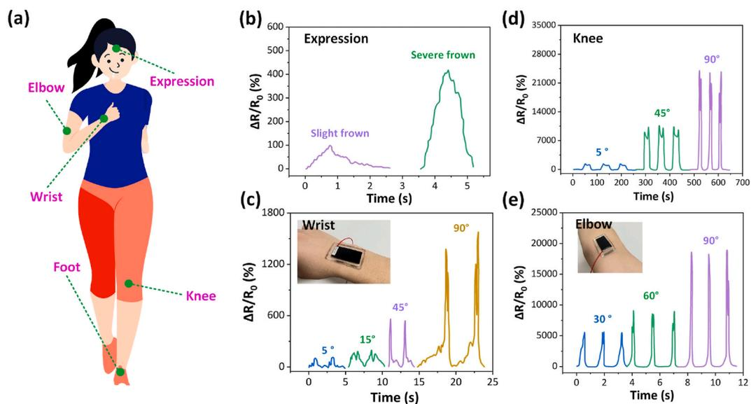
**Fig. 4.** (a) The performance photos of athlete. (b) The sensor signal of CC-strain sensor under athlete frown expression. The sensor signal of CC-strain sensor installed on (c) wrist, (d) knee, and (e) elbow at different bending angles of corresponding joints.
