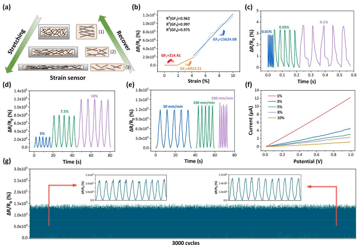
**Fig. 3.** (a) The sensing mechanism of CC-strain sensor device. (b) The relationship between  $\Delta R/R_0$  and strain. (c, d) The  $\Delta R/R_0$  signal of CC-strain sensor device under different strains. (e) The  $\Delta R/R_0$  signal of CC-strain sensor device under different loading speeds. (f) The I/V curves of CC-strain sensor under different strains. (g) The sensing stability test of CC-strain sensor device.
