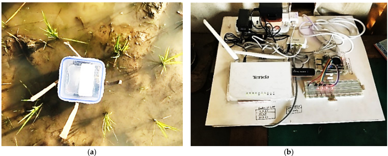
Figure 11. Agricultural field level trial setup: (a) Top view of a sensor device in the field (b) The receiver base station setup.
