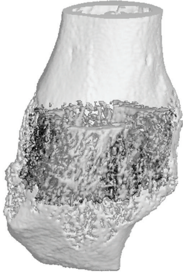
FIGURE 4: Hybrid \mu -CT image of the fracture region. The callous region is colored darker.
