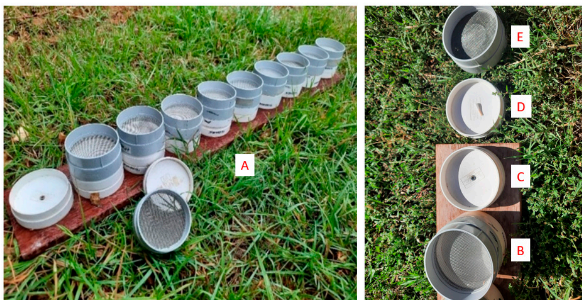
Figure 1. Scent board with 10 detachable PVC pots used in training (A). Each complete pot (B) consists of a base fitting (C) screwed to a timber board, a detachable tray fitting (D) into which an odor can be placed and a mesh cap fitting (E) which prevents access to the odor.
