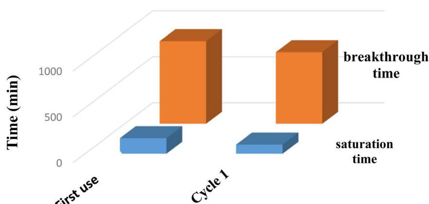
Fig. 7 Effect of the regeneration of the activated carbon bed  $Al(OH)_3@AC$  on the breakthrough and saturation times. Experimental conditions:  $[F^-]_0 = 10 \text{ mg L}^{-1}$ , volume flow rate =  $7.5 \text{ mL min}^{-1}$ , bed height = 3 cm, initial pH = 6.15,  $T = 22^\circ\text{C}$ .
