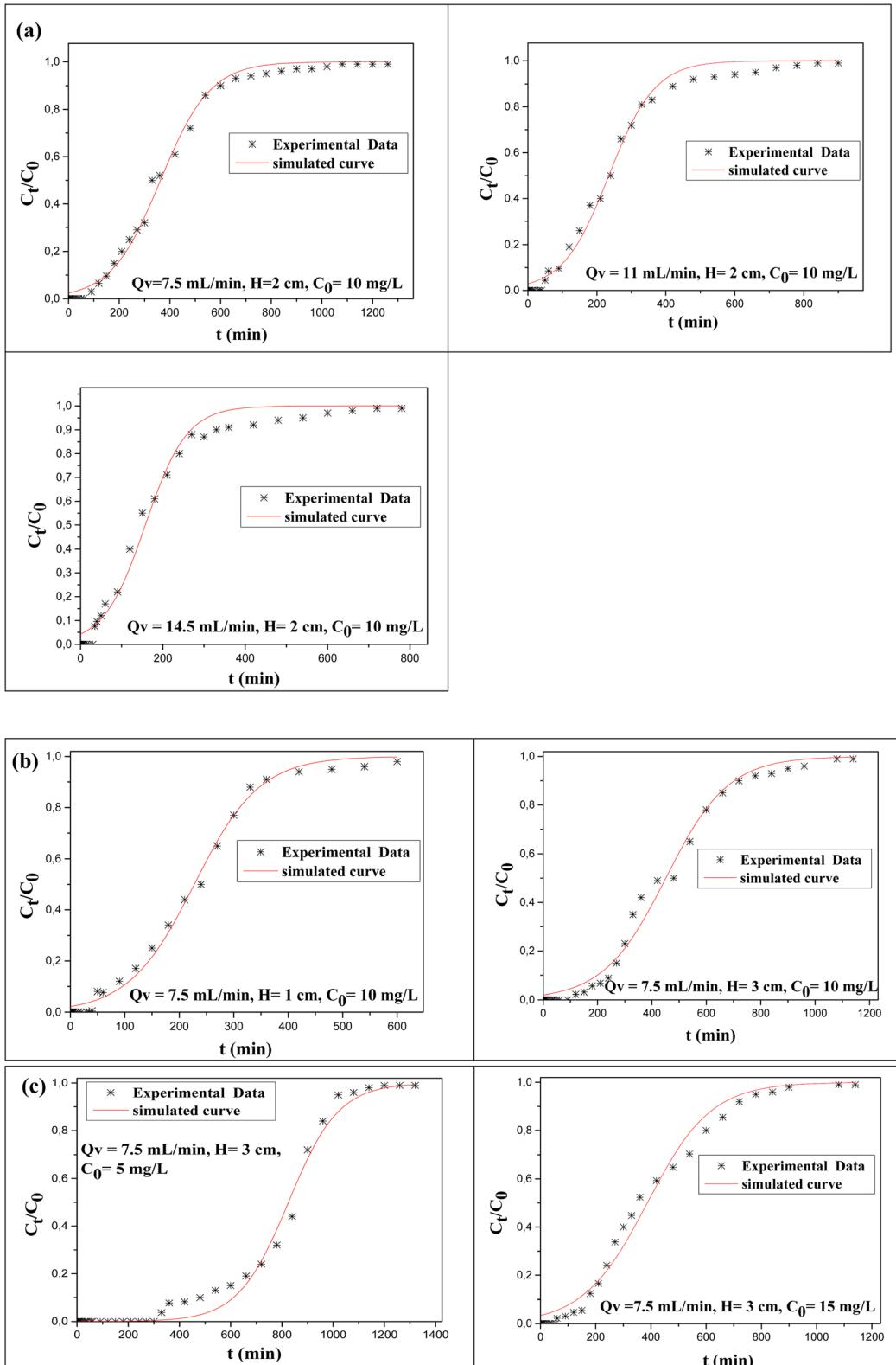
Fig. 4 Breakthrough, experimental and calculated curves obtained from the Yoon–Nelson model for different (a) flow rates, (b) bed heights, and (c) initial concentrations.
