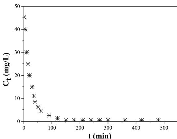
Fig. 6 Evolution of the concentration of fluoride at the outlet of the column as a function of time.  $[NaOH] = 0.01 \text{ mol L}^{-1}$ , bed height = 3 cm, flow rate =  $7.5 \text{ mL min}^{-1}$ ,  $T = 22^\circ\text{C}$ .
