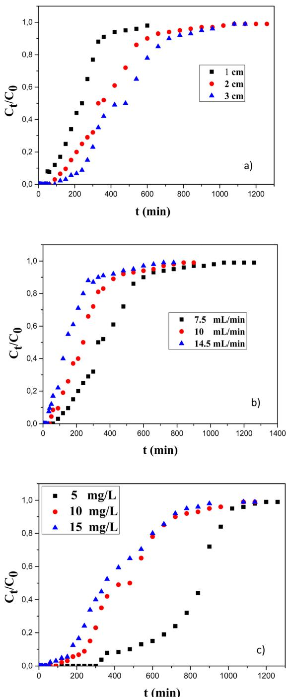
Fig. 1 Effect of (a) bed height, (b) flow rate and (c) initial fluoride concentration on breakthrough curves of fluoride adsorption on  $\text{Al}(\text{OH})_3@\text{AC}$  in the column system.
