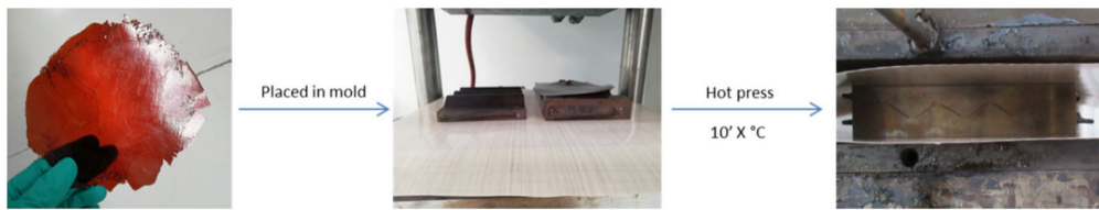
Figure 4. Procedure for reprocessing the prepared materials.
