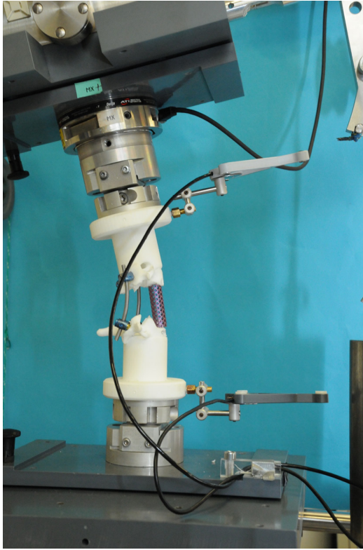
Fig. 1. The spine simulator with a 3-dimensional motion analysis system.
