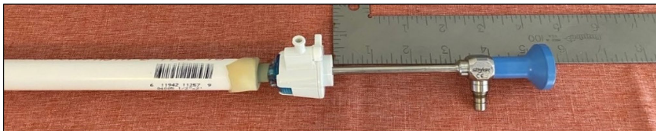
Fig. 2 Dynamic instrument–port interaction setup with 3 inch offset from full device insertion
