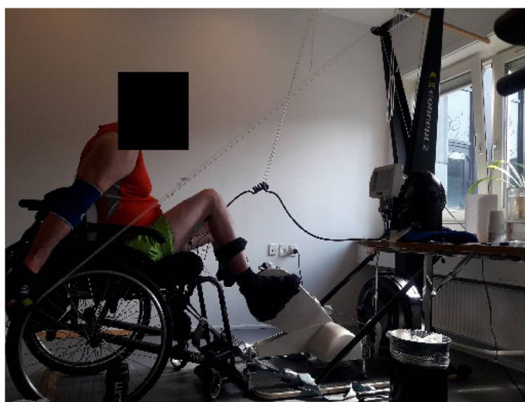
Fig. 1 The setup with the wheelchair positioned in front of RT300 FES leg cycle while pulling the Concept2 ski ergometer. Written permission to show photograph is given by the participant
