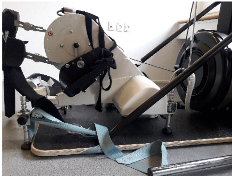
Fig. 2 The RT300 FES leg cycle positioned as close to the Concept2 ski ergometer as possible with two legs on the ski ergometer floor plate
