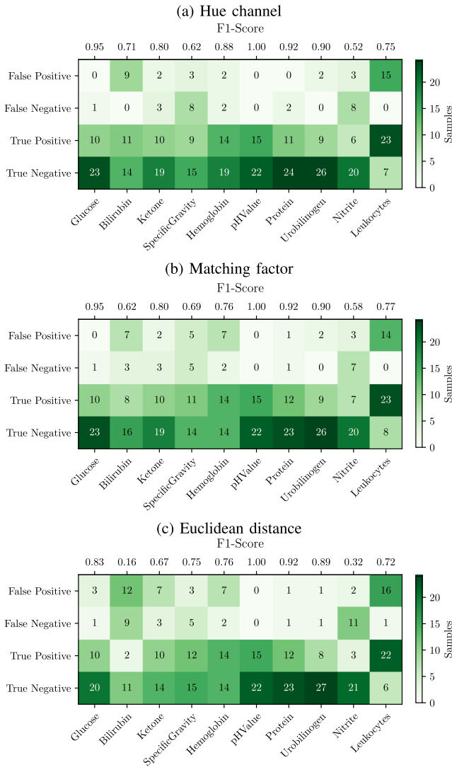
FIGURE 6. Confusion matrices of the automated urine test strip evaluation using three different methods: a) comparison of hue values, b) matching factor, c) Euclidean distance.
