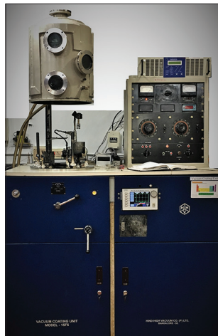
Figure 2: Vacuum-coating unit model, HINDHIVAC vacuum-coating unit model no. 15 F6 (Hind High Vacuum Co., Bangalore), helps in producing fine uniform, pure film coating of various metals
