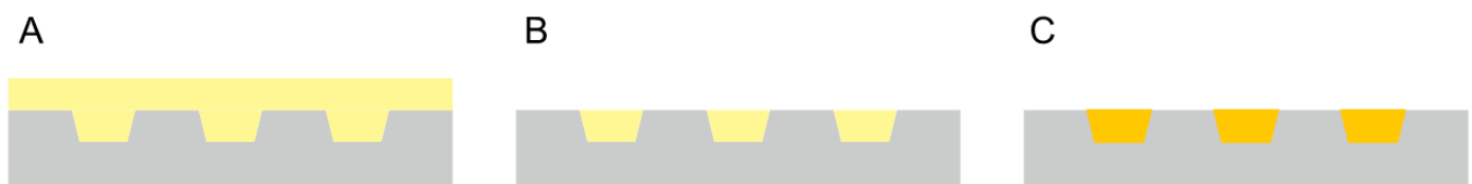
Figure 3. Fabrication process of the LGP-implanted chip. (A) LGP mixed with the main agent and crosslinker were deposited on the polystyrene microarray chip. (B) LGP on the microarray chip surface was removed. (C) Polymerization reaction of the LGP was performed at room temperature of 22 ^{\circ}\text{C} for over 24 h.
