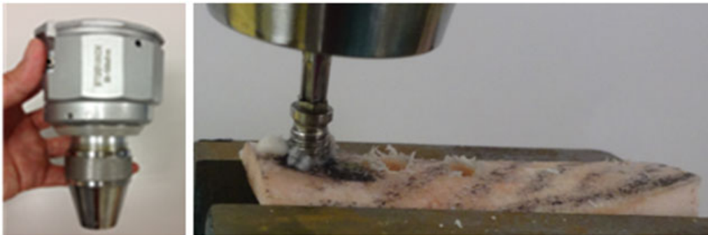
FIGURE 3 Digital torque gauge and regions of implantation. Ultrasound propagated the distal parts of the bone samples, and implants were inserted into the proximal, middle, and distal part of these parts
