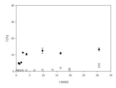
**Figure 4.** Comparison of biodiesel yield according to lipase origin (•—commercial lipase Lipolase 100L (Experiment 5), O—purified lipase produced by solid-state fermentation (Experiment 9)).
