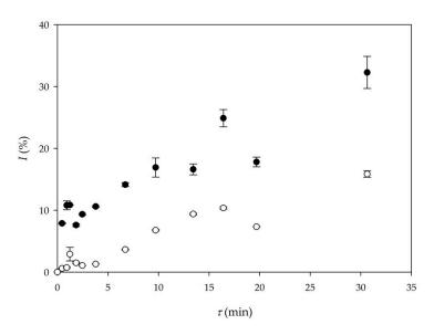
**Figure 3.** Comparison of biodiesel yield in different reaction mediums ( $\bullet$ —buffer as a reaction medium (Experiment 6),  $\bigcirc$ —DES as a reaction medium (Experiment 8)).
