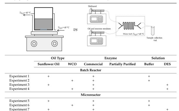
**Table 1.** Experimental setup and different reaction conditions during oil transesterification catalyzed by lipase performed in a batch reactor and in a microreactor system.
