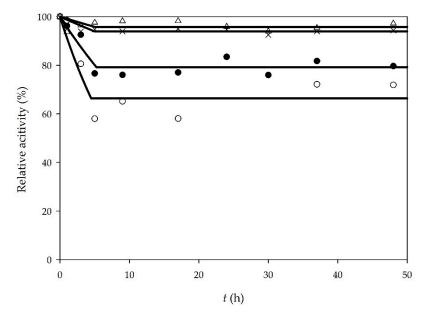
**Figure 1.** Lipase stability in batch processes ( $\bigcirc$ —edible oil, enzyme dissolved in buffer, •—waste oil, enzyme dissolved in buffer,  $\triangle$ —edible oil, enzyme dissolved in deep eutectic solvent (DES), ×—waste oil, enzyme dissolved in DES).
