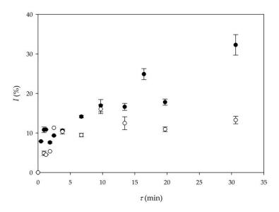
**Figure 2.** Comparison of biodiesel yield depending on oil origin (O—edible oil (Experiment 5), •—waste cooking oil (WCO) (Experiment 6)).
