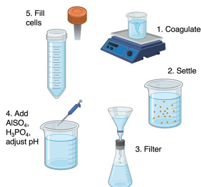
Figure 1. Summary of test water preparation for the coupon study (created at biorender.com ).
