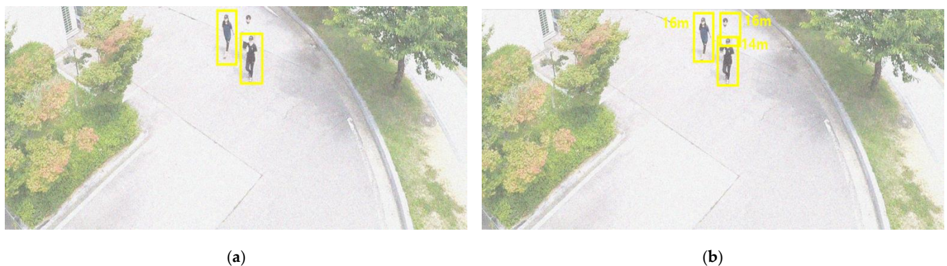
Figure 10. Comparison of pedestrian detection results by vision-based faster R-CNN (a) and RGDNet (b).
