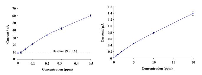
**Figure 10.** Free chlorine calibration curve; "Low" range 0 to 0.5 ppm (Mean RSD 3.8%), "High" range free chlorine calibration curve from 0 to 20 ppm (Mean RSD 4.2%).
