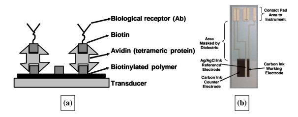
We successfully utilised this approach to construct immunosensors for the antibiotic ciprofloxacin which could detect levels of 1 ng mL<sup>-1</sup> of the antibiotic, not only in PBS [62] but also in milk [63]. We have also developed electrochemical immunosensors for myelin basic protein—a marker for stroke and multiple sclerosis [64] and Internalin B, a surface protein marker for Listeria [65].
