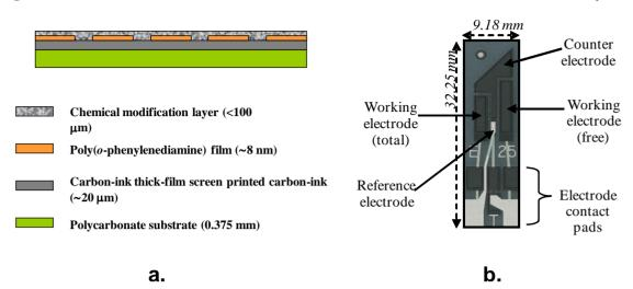
Figure 8. (a) Schematic of final sensor construction; (b) final four-electrode assembly.
