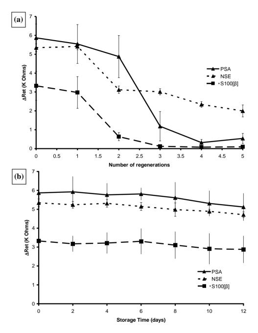
Samples of all three immunosensors were stored dry at 4  $\,^{\circ}$ C for up to twelve weeks and two of each tested at two week intervals. As Figure 25b shows, the performance did not deteriorate with storage. Samples containing embedded PSA were also tested, and were found to be stable for up to six weeks but after 12 weeks their performance had deteriorated to about a third of "fresh" sensors [66].
