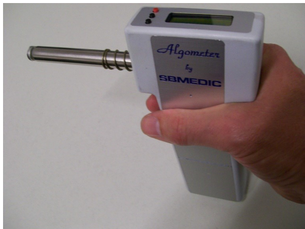
Fig. 1. Picture of the deep tissue pressure algometer with electronic force gauge (Algometer II®, SB-Medic, Sweden) used in the study.
