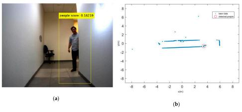
Figure 1. (a) Detected moving person; (b) His extracted depth from laser sensor.
