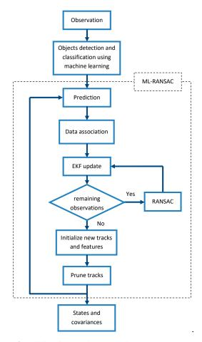
**Figure 3.** Overall scheme of multilevel-RANdomSAmple Consensus (ML-RANSAC) algorithm for Simultaneous Localization and Mapping with multi-target tracking (SLAMMTT).
