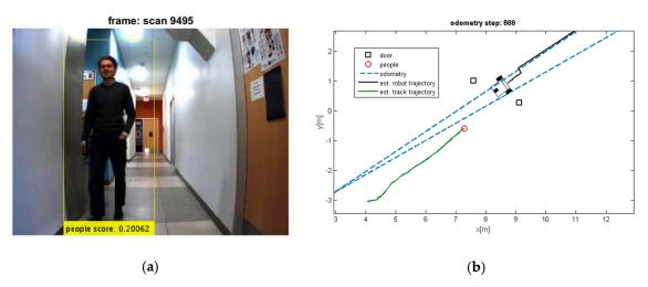
**Figure 10.** (a) Detected moving people; (b) Estimated trajectories of robot and tracks along with the estimated position of doors.
