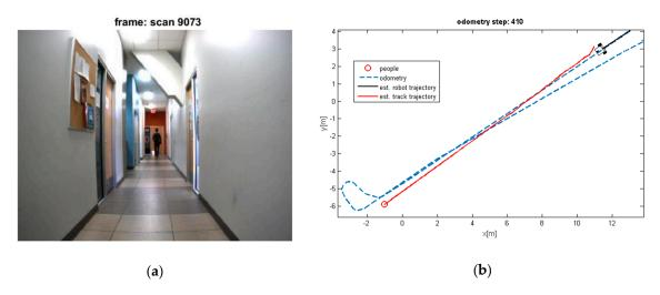
**Figure 9.** (a) Losing the detection of moving people; (b) Estimated trajectories of robot and tracks, whereas the proposed algorithm keeps tracking the moving object.
