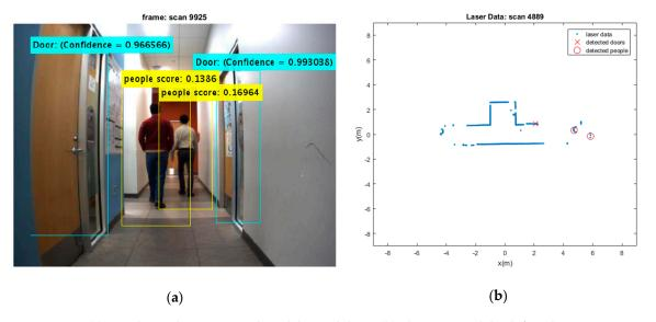
Figure 7. (a) Two detected moving people and detected doors; (b) Their extracted depth from laser sensor.
