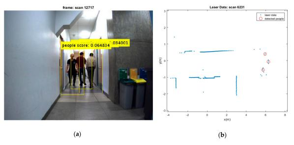
Figure 6. (a) Three detected moving people; (b) Their extracted depth from laser sensor.
