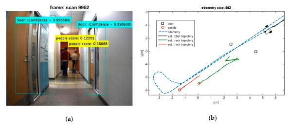
**Figure 11.** (a) Detected moving people and detected doors; (b) Estimated trajectories of robot and tracks along with the estimated position of doors.
