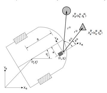
Figure 4. Vehicle and observation kinematics [38].
