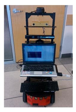
Figure 5. Pioneer P3-DX mobile robot with mounted sensors.
