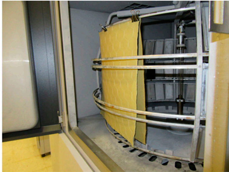
Figure 3. Exposing fabrics in the Atlas weather-ometer Ci-5000.
