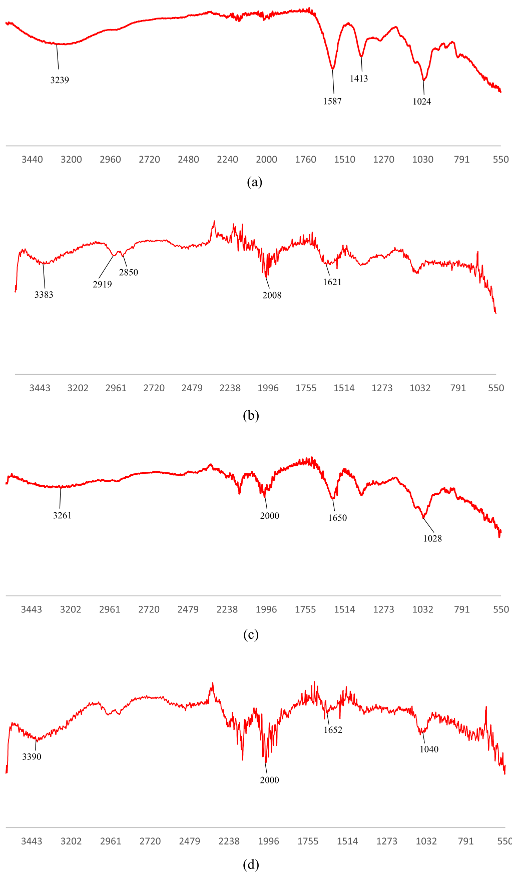
Figure 5. FTIR spectra of ALC (a), SLAC (b), SLACC before adsorption (c), and SLACC after adsorption (d).
