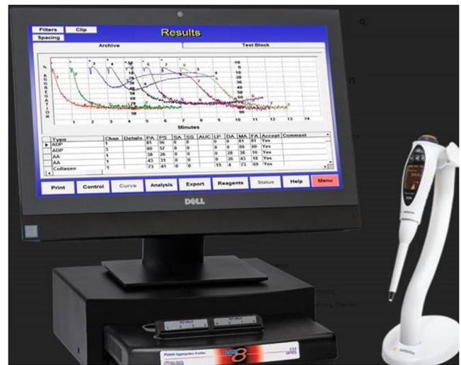
FIGURE 1 PAP-8 light transmission aggregometer (Bio/Data Corporation): This system measures the rate and extent of platelet aggregation, agglutination, and activation stimulated by individual agonists; platelet agglutination/aggregation is indicated by degree of light transmission.
