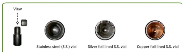
Figure 4. Milling vessels lined with copper and silver foil demonstrated by the Mack group. [6b] Published by The Royal Society of Chemistry.
