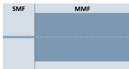
Figure 2. Single-mode fiber (SMF)-multimode fiber (MMF) structure used in the simulations to illustrate the main features of multimode interference (MMI) devices.
