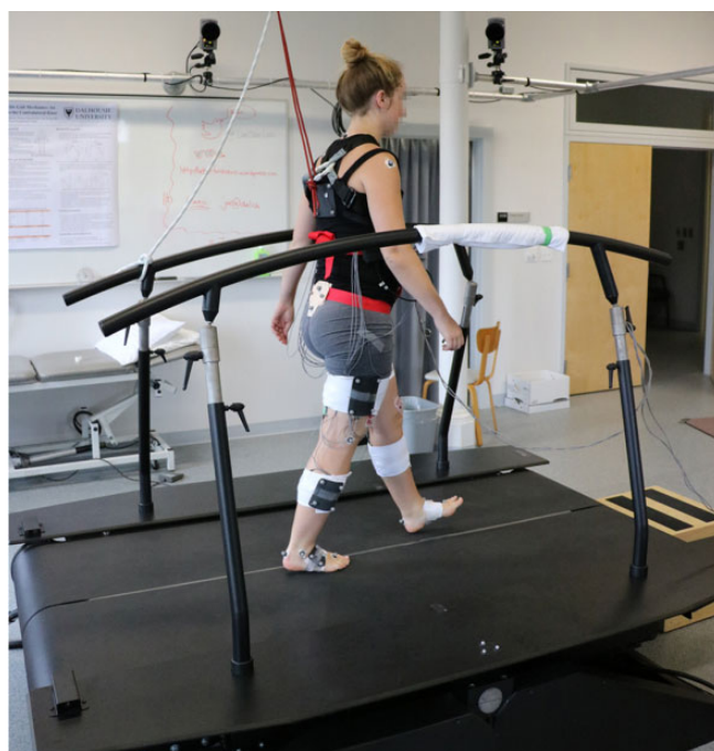
Figure 1. Image of a participant walking atop the dual-belt instrumented treadmill as part of this study. Markers shown are those tracked during walking, including a rigid plate on the pelvis, femur, shank, and foot and single markers placed on the shoulder, lateral epicondyle, lateral malleolus, calcaneus, and second metatarsal bilaterally. Electrodes are located as described in Table 1 and have been covered with tensor wrap.
