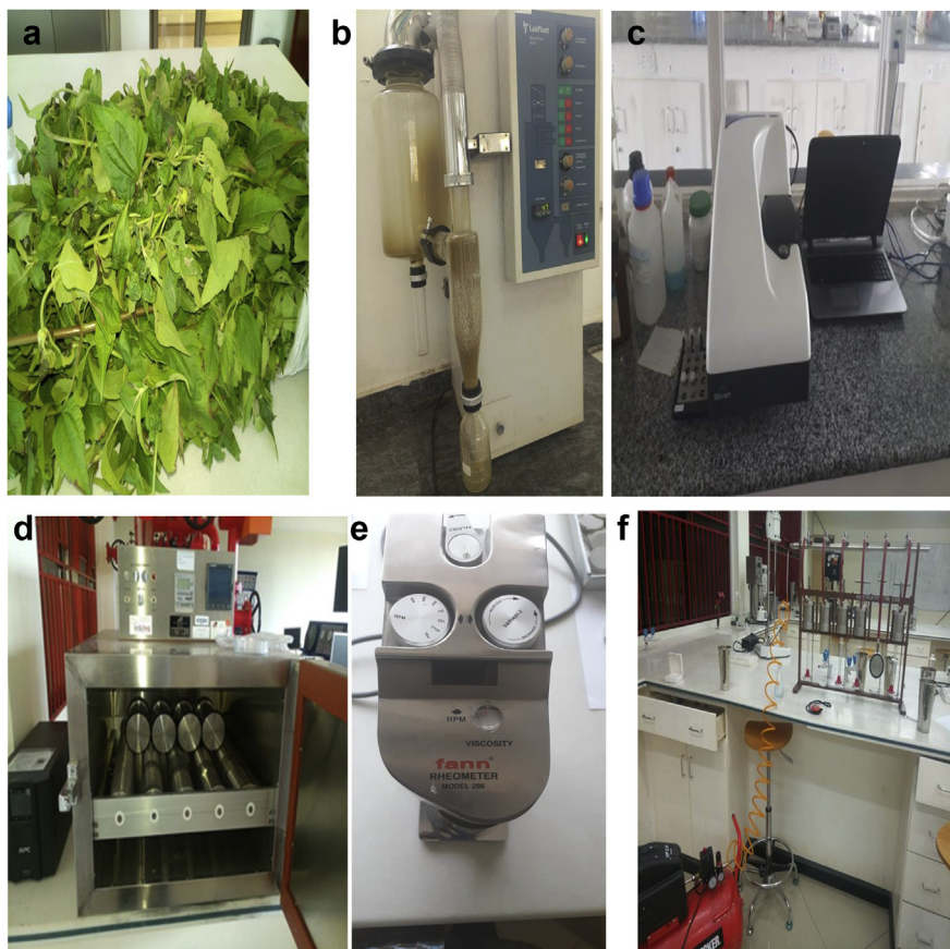
Fig. 1. a) Chromolaena odorata Leaf Collected for Analysis. b) Lab Plant SD-05 Spray Dryer used for test. c) Malvern Zetasizer Nano ZS90. d) 5-Speed Hot Roller Oven. e) FANN Rheometer model. f) API Low Pressure Multiple Filter Press.
