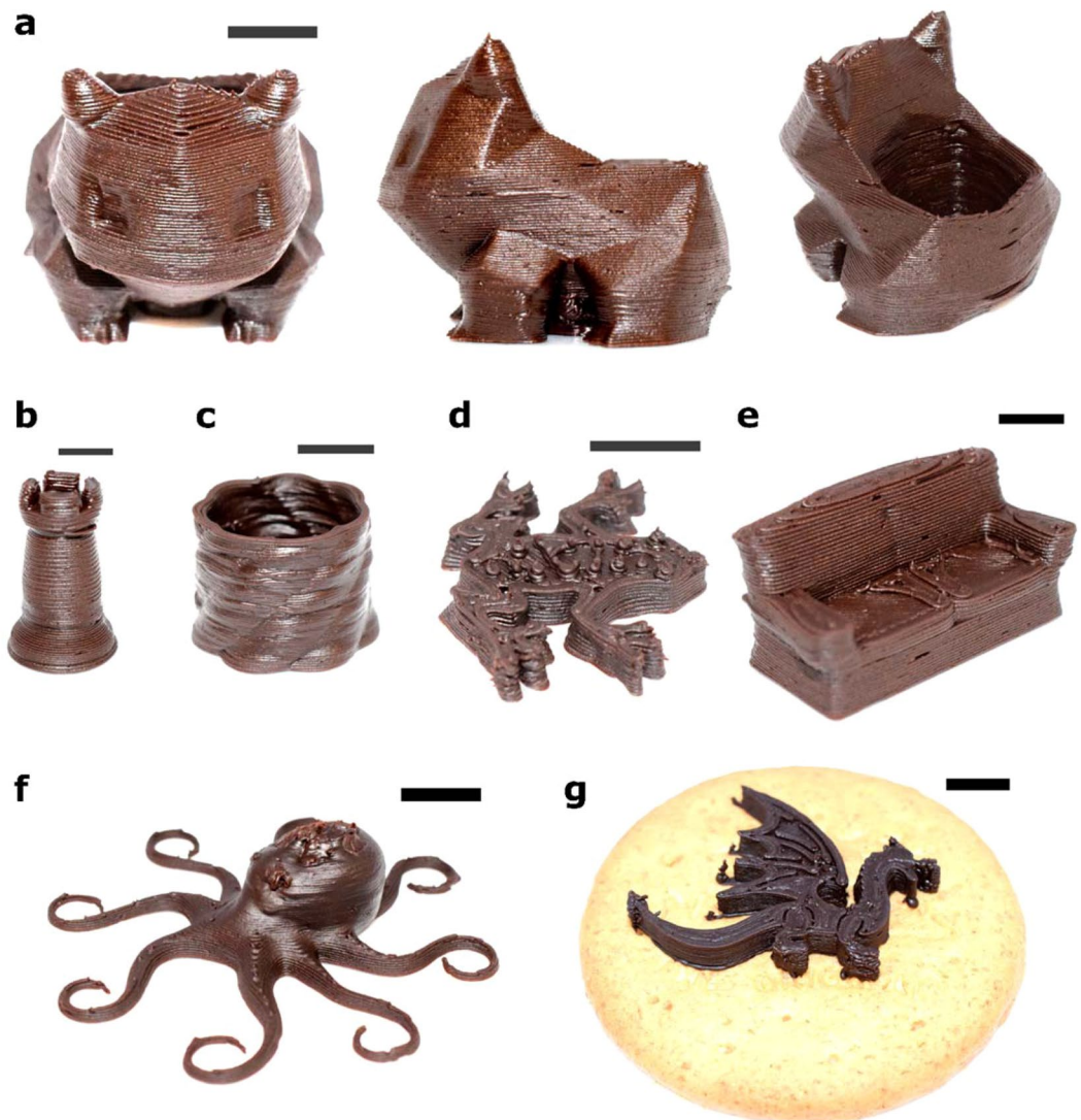
Figure 6. Optical images of 3D printed structures printed by direct chocolate-based ink 3D printing. (a–f) 3D structures of chocolate-based materials, printed with S20 and S25. (g) A 3D structure, printed with S20, of dragon directly printed on a biscuit as an underlying substrate. Scale bars = 1 cm.
