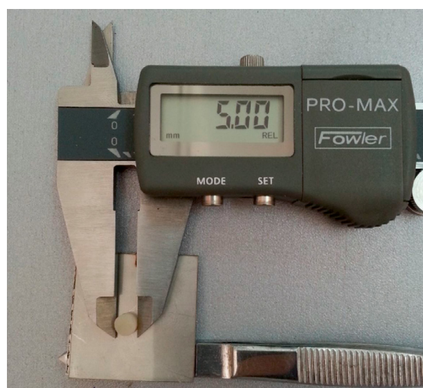
Figure 3- Compression test sample
