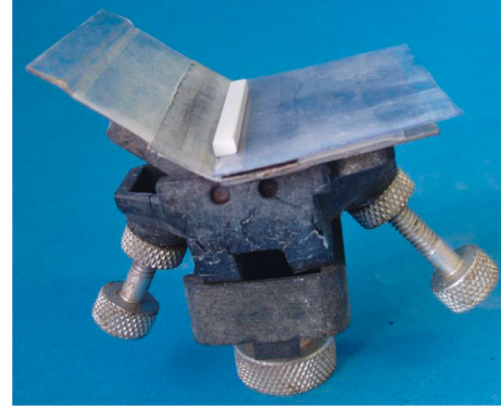
FIGURE 1: Setup to prepare the specimen 4-point bending chamfer on the edges.
