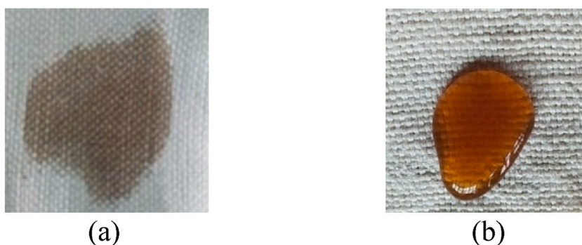
Fig. 4. Dropping liquid in the untreated fabric and (b) Dropping liquid in the treated fabric.
