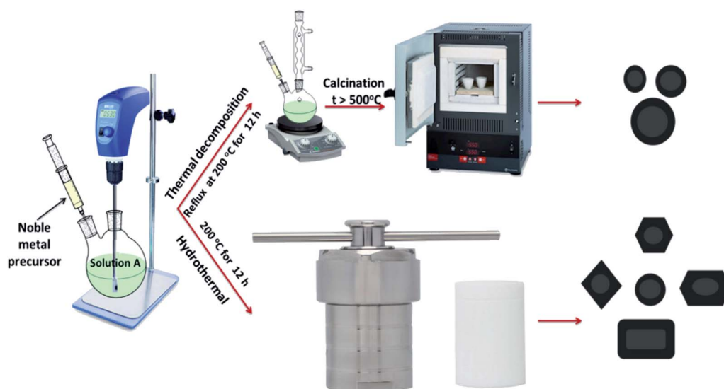
Scheme 1 Schematic representation of the procedures for the synthesis of Fe 3 O 4 @Ag and Fe 3 O 4 @Au core-shell NPs by the two methods.
