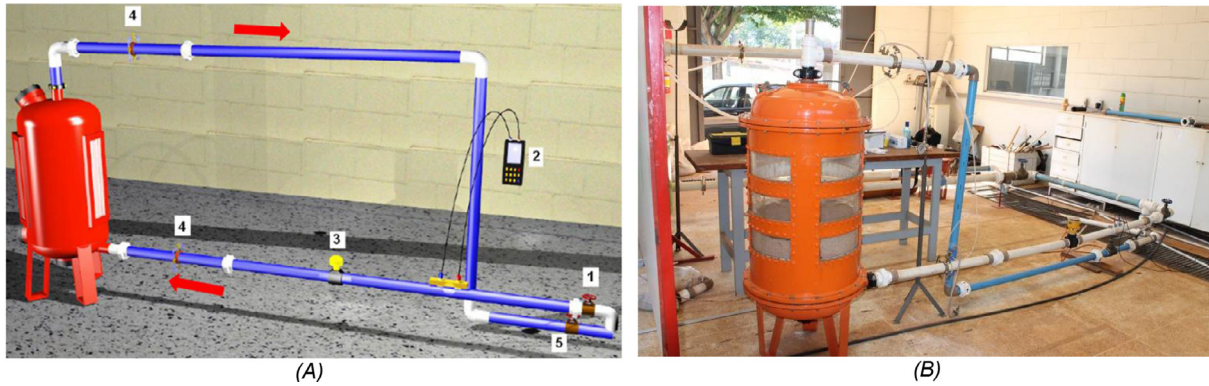
Fig 2. Diagram of the experimental module assembly with sand filters in a closed flow circuit, detailing the position of the equipment used in the experiment and the flow direction (1 and 5 – needle valves inlet and outlet respectively, 2 – ultrasonic flow rate, 3 – electromagnetic flow rate, and 4 – integral pressure sensors) (A), and a photo of the experimental module assembly (B).
