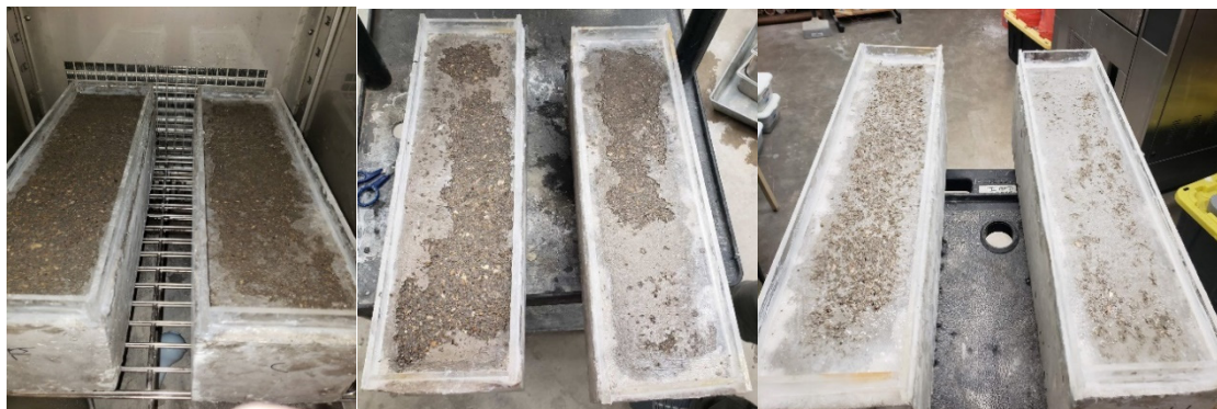
Figure 8. Scaling of concrete surfaces at 20 cycles (left to right: F20, C20, OP-0, OP-1, PL-0, PL-1).
