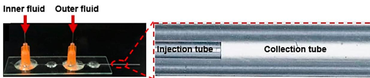
**Figure 9.** Microfluidic device with a co-flow structure developed by Xia et al. Reprinted from an open-access source [58].
