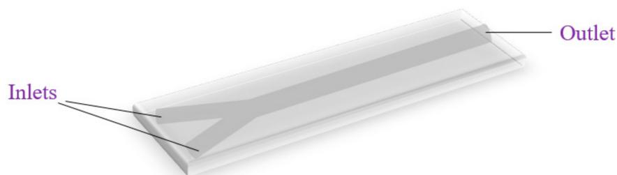
**Figure 4.** Schematic representation of a typical Y-type microreactor.
