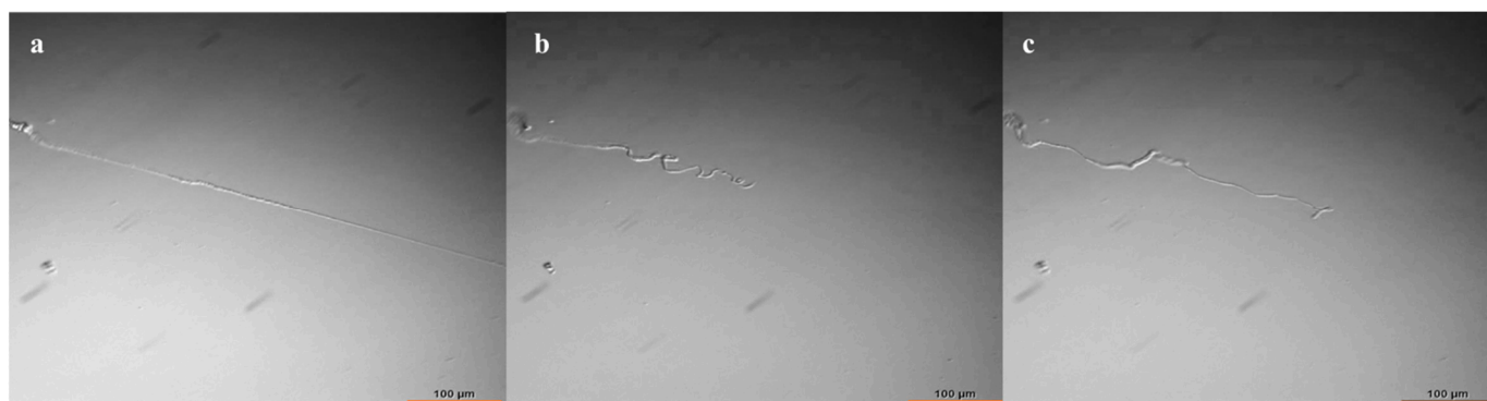
Figure 3. Optical microscopy images of (a) PAA( \text{Na}^+ ) thread expanded in water, (b) PAA thread contracted with \text{CaCl}_2 and (c) PAA thread re-expanded with ATP. Scale bar 100\text{ }\mu\text{m} .
