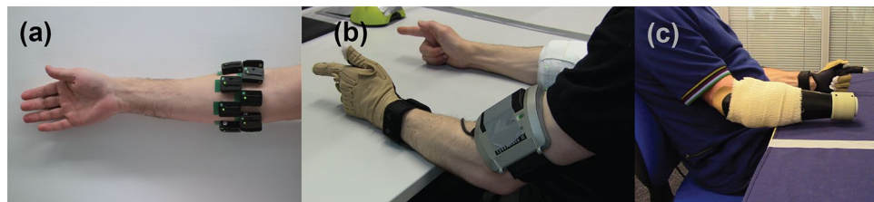
Figure 5. Data collection. (a) Sixteen wireless EMG sensors were placed on the surface of the skin and were arranged in two rows of eight equidistant sensors below the elbow. (b–c) Hand kinematic data were collected using an instrumented data glove placed on the contralateral side. Participants were instructed to perform bilateral mirrored movements. Parts of the figure were previously published by us under a Creative Commons Attribution License (CC BY 4.0) 21 .
